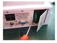
3. Pull the battery out until the plug connector system is completely out of the panel.
