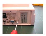
2. Pull the battery out of the panel by means of a screwdriver. **Attention!!** Do not poke the screw driver into the battery and do not drag it out forcibly.
