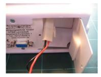
4. Press the locking device clip until the catch releases the counter piece, then disconnect the plug connector system. Then you can change the battery. The assembly is carried out in a retrogressive operation sequence from picture 4 to picture 1.
